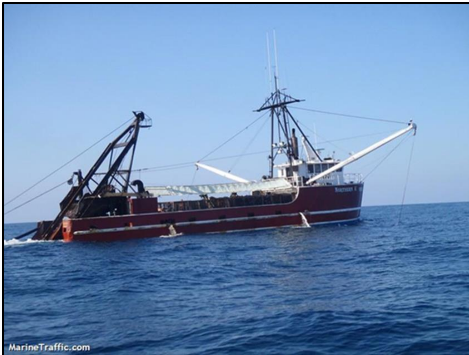
Figure 2.18 Hydraulic clam dredge fishing vessel in operation
